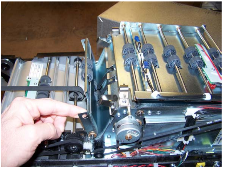
Transition baffle View
